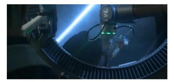
Similarly, we enhanced the reliability of our sealant application process for booster vane assemblies by leveraging automated sealant application machines. The automated process achieves high levels of
