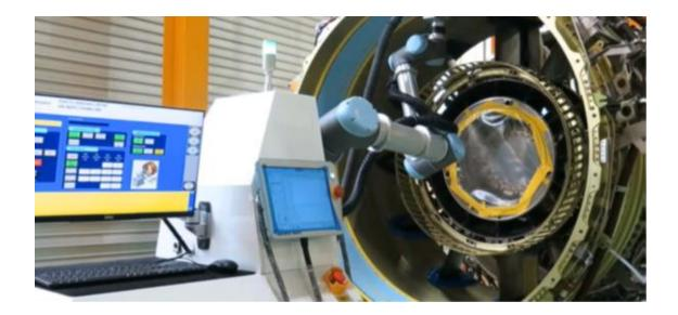
For instance, we have installed automated fan frame abradable machines in our shopfloors for the removal of worn abradable seals on engine fan frames. This increases precision in removing old seal materials and ensures a higher level of accuracy and reliability in the process, significantly improving the quality of maintenance for engine fan frames. This shift in workflow also resulted in a 500% increase in productivity, brought about by a reduction in manhours.
