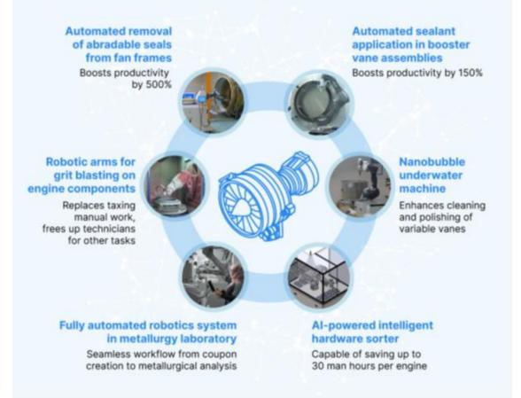
We are also leveraging nanobubble underwater technology in place of manual polishing for the servicing of compressor stator vanes to eliminate exposure to hazardous dust, a byproduct of the repetitive polishing process. We use automated robotic arms to immerse these vanes into a water tank, which then generates nanoscale bubbles. The bubbles clean and polish the vanes at the same time, resulting in a more efficient workflow with higher-quality outcomes.
