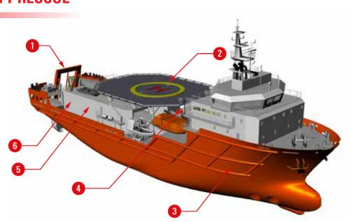
The Submarine Support and Rescue Vessel (SSRV) is designed and built for rescue operations of a distressed submarine. Operable up to sea state 5, the vessel is highly manoeuvrable and has good speed and seakeeping performances.
